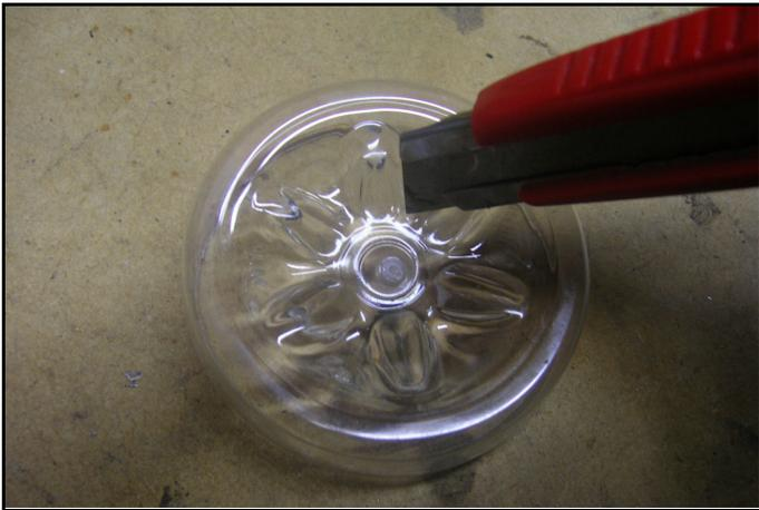
Either cut or drill a hole in the end of the bottle that you cut off earlier. The hole must be big enough to fit the tube of mesh through.
