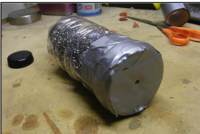
Wrap some duct tape around it to secure it altogether plus a few layers around the front. The idea is to fire a bullet through the tape to make the exit hole. The first shot will always be quieter but you can always just put another bit of fresh tape over the hole.
