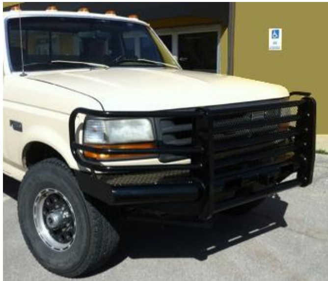
Heavy Duty bumper/Elk Guard and running lights added to the truck
